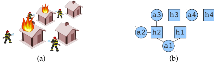
Figure 1: (a) Illustration of an MPOMDP in which a team of agents has to fight a fire, and (b) Illustration of the coordination graph (as a factor graph) with houses represented as h_1, \dots, h_4 and agents represented as a_1, \dots, a_3 . Each agent should coordinate with the adjacent agents in the graph.
